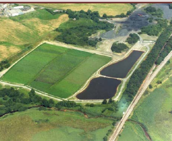
Fig 2. Aerobic treatment systems in South Wales. Morlais (5 hectares) and Taff Merthyr (4 hectares) are some of the largest constructed. 2
