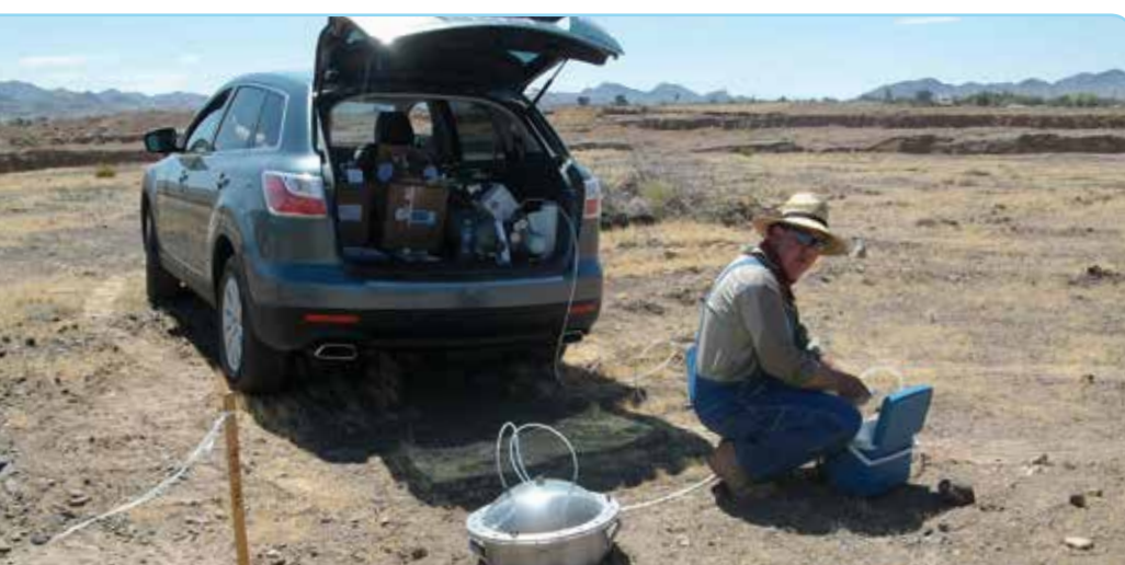
Installing a USEPA flux chamber
