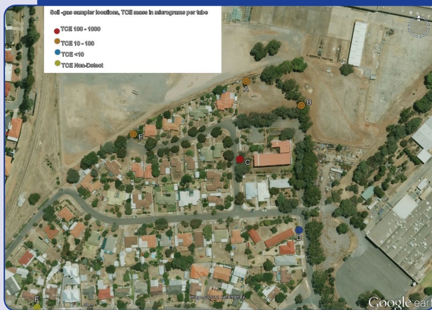
Figure 1. Locations of passive soil vapour sampling sites within the residential study area. The colours of the sample locators indicate the mass-range of TCE adsorbed onto the Radiello® passive samplers at a sample depth of 2 metres.
