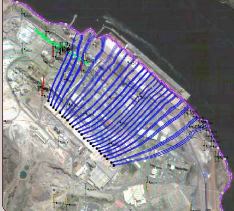
FIGURE 5 The calibrated flow and particle tracking model.
